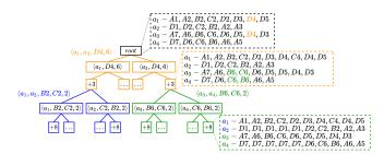
Figure 4: A CT for solving the MAPF instance in Figure 1 with MA-CBS.
