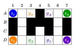
Figure 1: An illustrative 4-agent MAPF instance. Each start vertex  $s_i$  of agent  $a_i$  is shown as a solid circle, while its goal vertex  $g_i$  is shown as a hollow circle in the same color.
